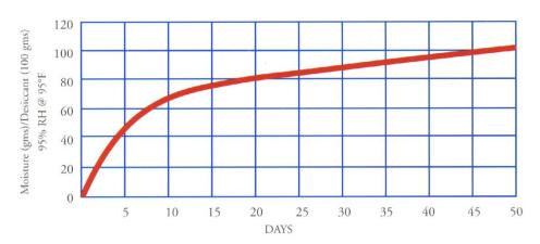
This graph depicts CARGO DRYPAK absorbing over 100% of its weight in moisture. CARGO DRYPAK will continue to absorb moisture for over 50 days inside standard shipping containers.
