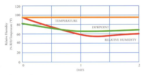
This graph illustrates CARGO DRYPAK reducing the dewpoint and relative humidity inside a standard shipping container at (95% RH@95°F). By reducing the dewpoint, CARGO DRYPAK prevents condensation from forming for over 50 days.
